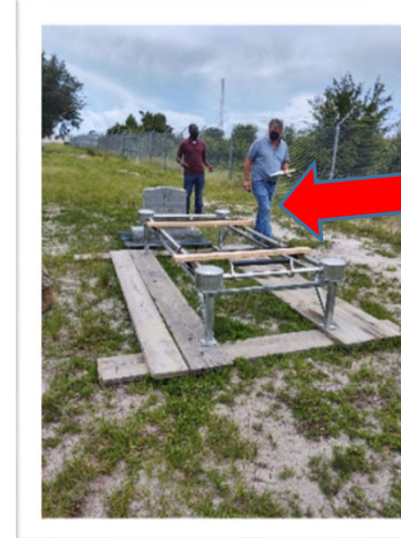
BODY BEARER 70"W x 100" D x 23" H INCLUDE A 61 FOOT AREA ONE SHORT SIDE
