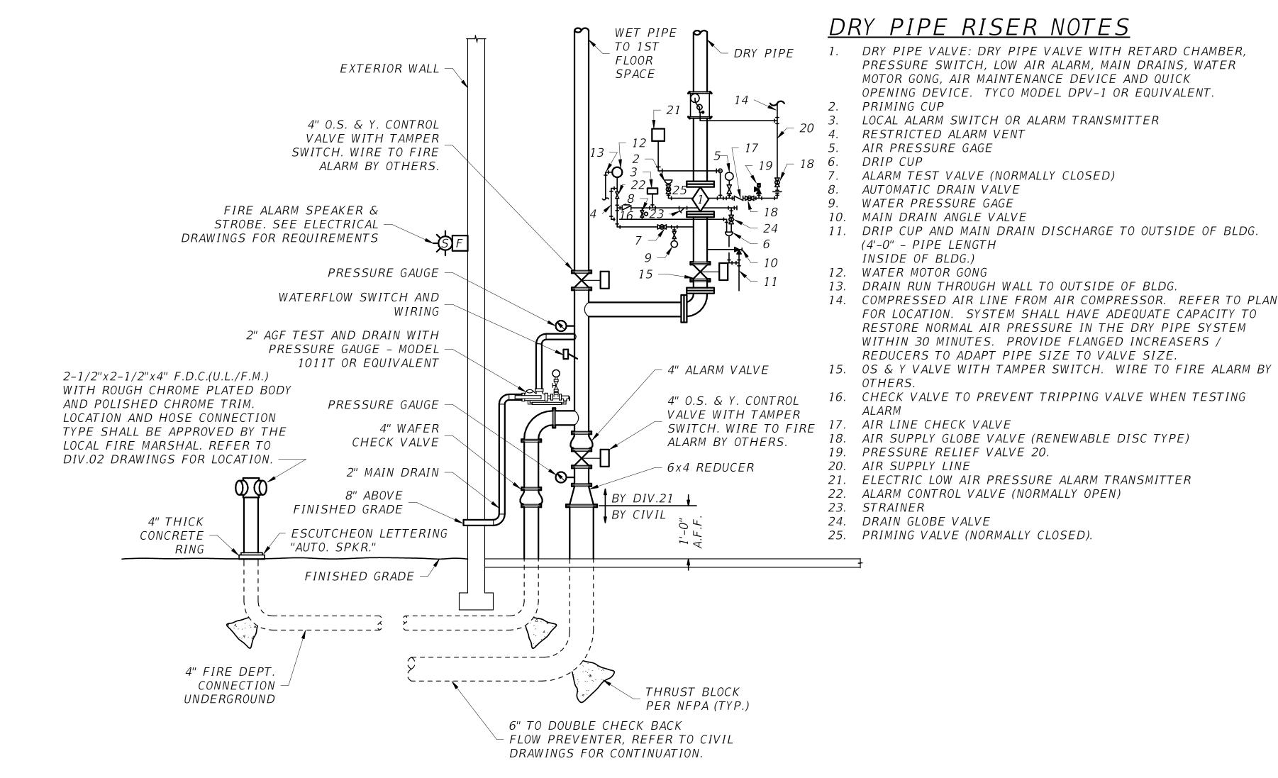
COMBINATION WET AND DRY PIPE RISER DETAIL NOT TO SCALE
